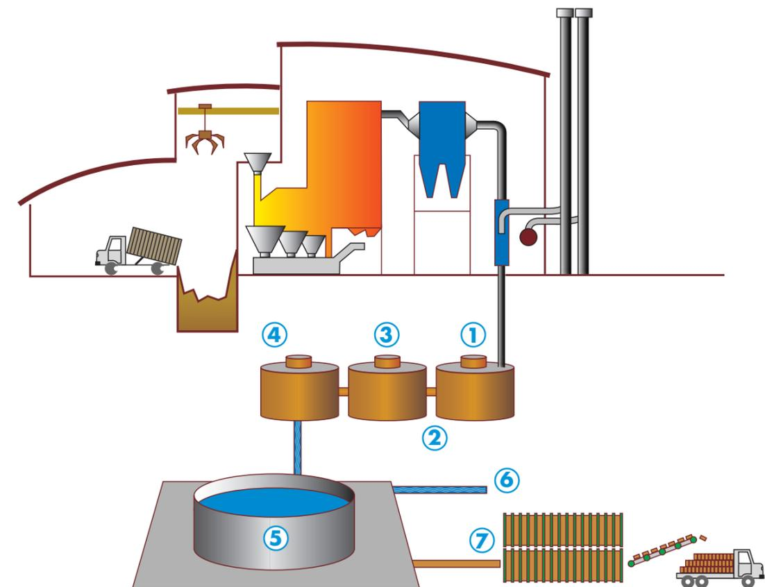
**1. Lime or caustic pretreatment** : neutralisation and hydroxide precipitation of the wastewater coming from the scrubber
